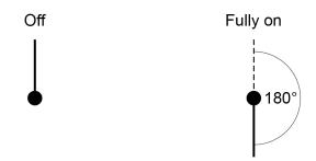
When fully on, water flows out of the tap at 14 litres per minute.
